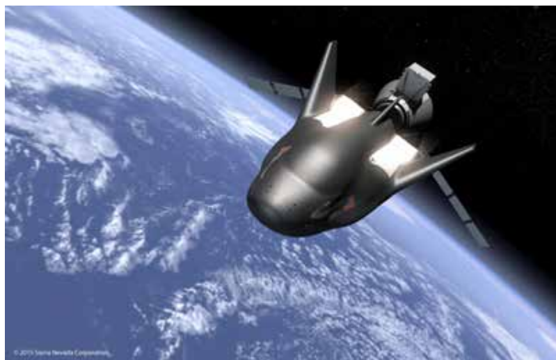
An artist's concept of Sierra Nevada's Dream Chaser mini-shuttle in orbit. A disposable rear cargo module has just separated. While the shuttle will return with cargo to Earth for reuse, the cargo module will burn up in the atmosphere. (Sierra Nevada Corporation)
