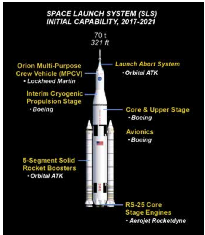
The hodge-podge of contractors involved in building SLS. Adapted from 2012 NASA PowerPoint presentation. (NASA)
