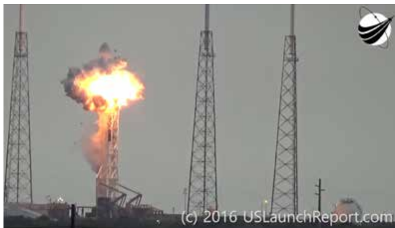
On September 1, 2016 a Falcon 9 rocket with a commercial payload exploded on the launchpad during a prelaunch dress rehearsal of the countdown. This failure and the ensuing investigation canceled all of SpaceX's planned launches in 2016. (USLaunchReport.com)
