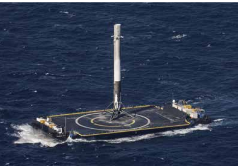
The Falcon 9 first stage sits intact after completing the first-ever vertical barge landing on April 8, 2016, during the launch of a Dragon capsule to the International Space Station. (SpaceX)
