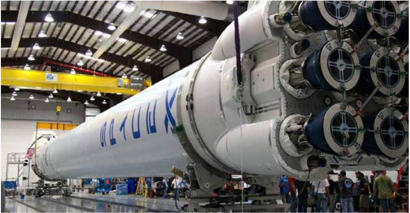
An early Falcon 9 rocket awaits launch in October 2012. Note the square arrangement of the nine Merlin engines, later changed to a circular pattern. Note also the lack of landing legs, which were added later. (SpaceX)
