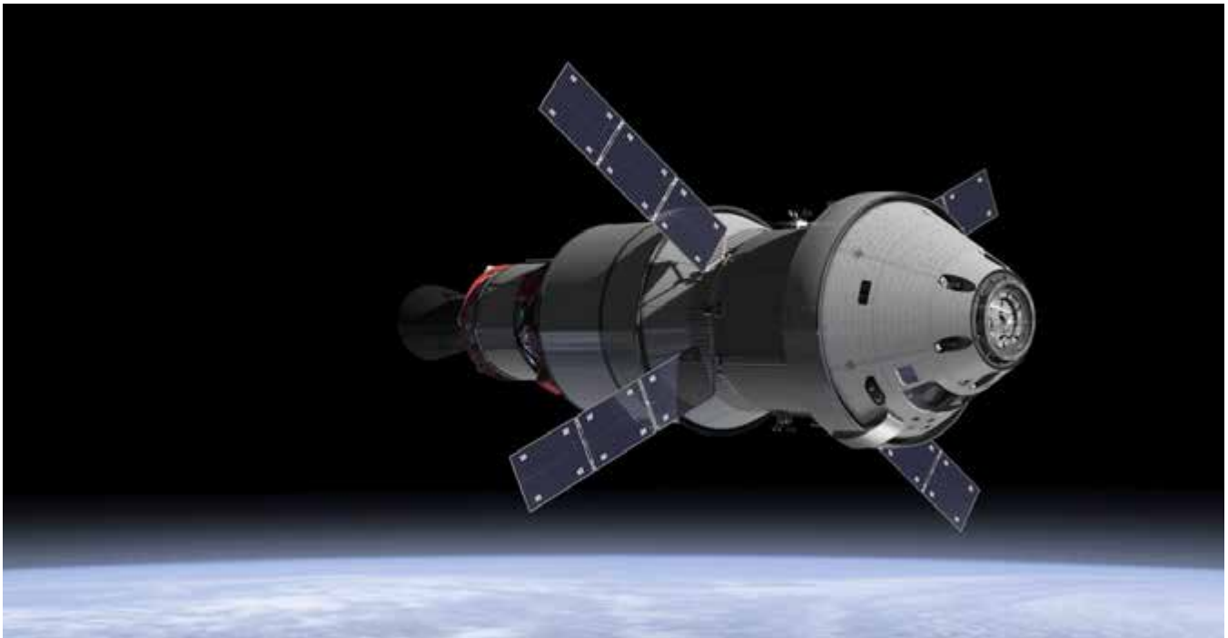
An artist's concept of the European Space Agency's service module, attached to the Orion capsule. (NASA)
